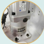
SERVO MOTOR WITH REDUCER
